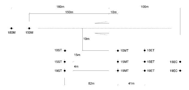
The ramp must be parallel to the jump course and slightly open. The tolerance for standard jumping is between +1.00° and +2.50° open. The tolerance for ski flying is between +5.00 and +7.00 open. Open means that the low end of the ramp is turned toward the jump course. The basis of the jump course is the 15ST-15MT line.
